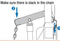
6. Insert Snapper Pin then Raise Drop Foot
