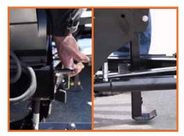
**Optional Wings -** Part No. | 16021712 Add a full 2' of width to your plow with the VXF Series Plow Wing Kit.
