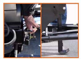
**Optional Wings -** Part No. | 16021610 Add a full 2' of width to your plow with the EX Series Plow Wing Kit. Wings rotate behind plow for easy stowage, no lifting required. Pin shears upon impact to protect from damage.
