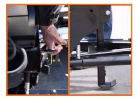
**Optional Wings -** Part No. | 16021510 Add a full 2' of width to your plow with the HD Series Plow Wing Kit. Wings rotate behind plow for easy stowage, no lifting required. Pin shears upon impact to protect from damage.
