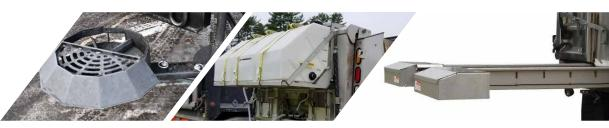
Telescopic spinner provides options to adjust material placement.
