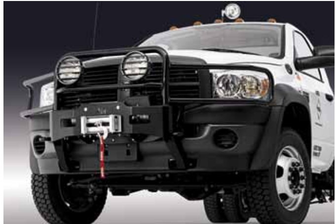
The Gen II Trans4mer System can be configured in a variety of ways. It can be as simple as a place to mount a winch (right) or highly customized with the array of optional accessories (left).
