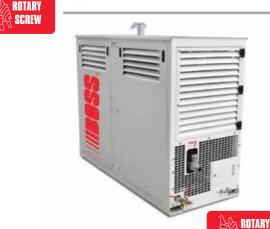
This diesel driven 74hp T4F John Deere engine and skid mounted rotary screw air compressor is rated at no less than 210cfm at 100psig for our 210 DUS and 250cfm at 100psig for our 250 DUS. The heavy duty design is perfect for OEM truck mounted applications.
