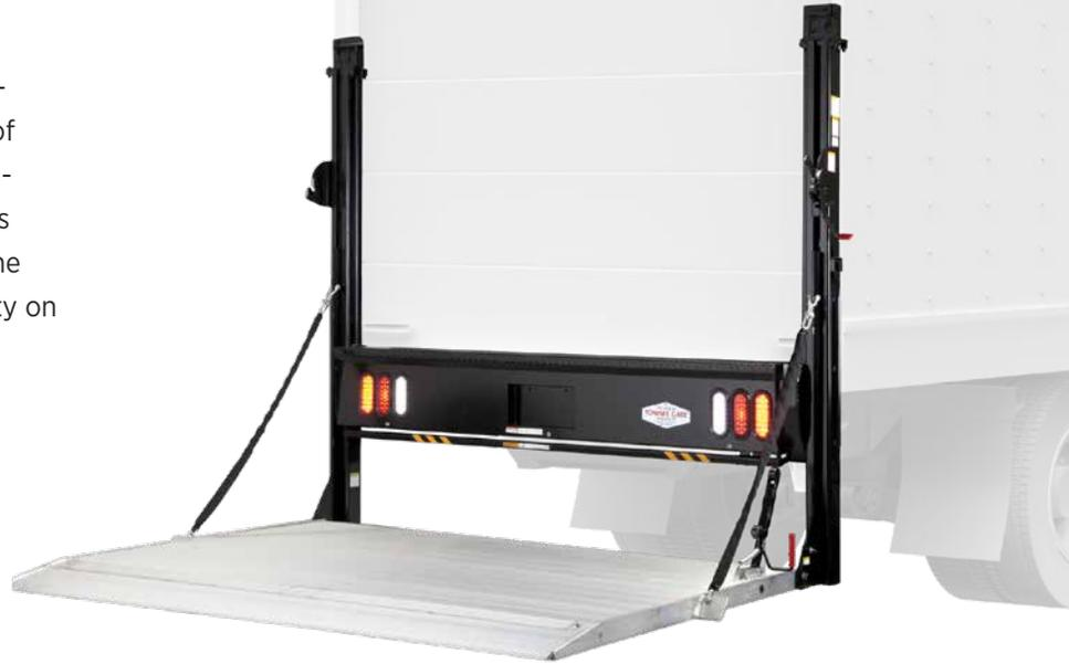
High-cycle railgates come standard with safety trip bar, auto open and close, and recessed lights. Taper-integrated cart stops are optional on extruded-aluminum platform models.
